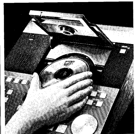
Top-loader with compartment for normal CDs and 8 cm singles
